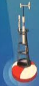
NOAA TAO Array Buoy (Tropical Atmosphere Ocean)
